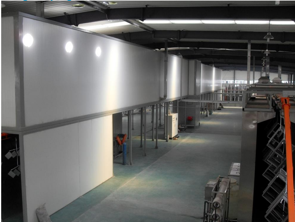
Bridge drying tunnel
